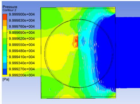
Figure 10: Distribution section of the air disturbance around the foil.
