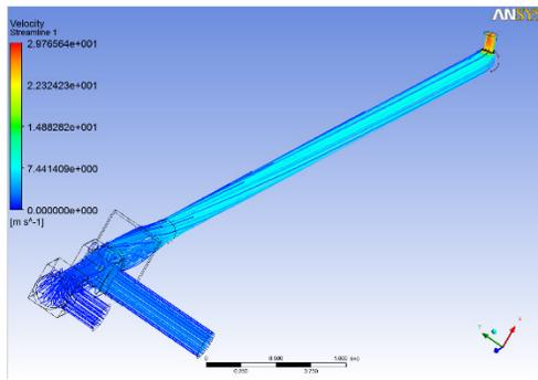
Figure 9: Separation of airflow of the stripper foil system.
