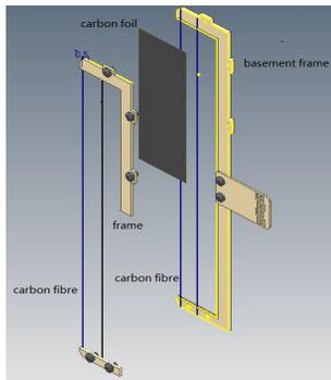
Figure 4: Bilateral fixed form of stripper foil.
