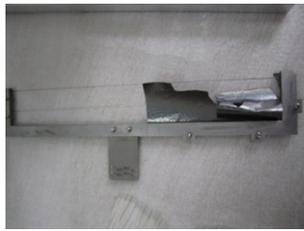
Figure 3: Broken experiment of CSNS stripper foil.
