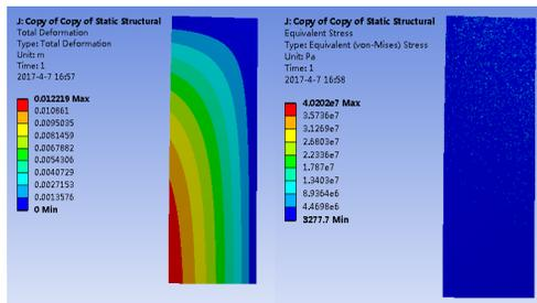
Figure 12: Stress and strain distribution on the foil.
