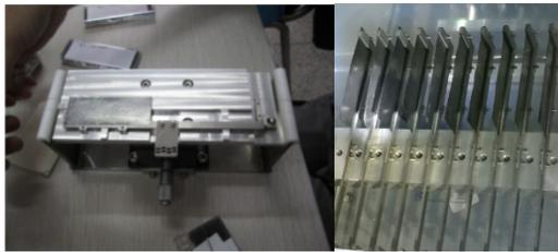
Figure 5: Stripper foil installation set and the samples.
