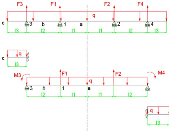
Figure 5: Force diagram of 4 support points beam.
