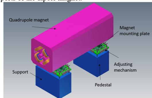
Figure 2: Quadrupole magnet supports.
