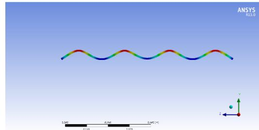
Figure 7: Deflection distribution of optimized support locations of slender beam.
