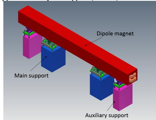
Figure 1: Dipole magnet supports for each module.
