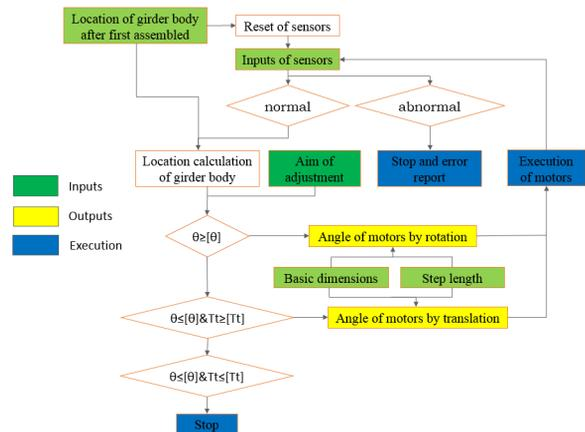
Figure 5: Flow diagram of the girder adjusting algorithm.
