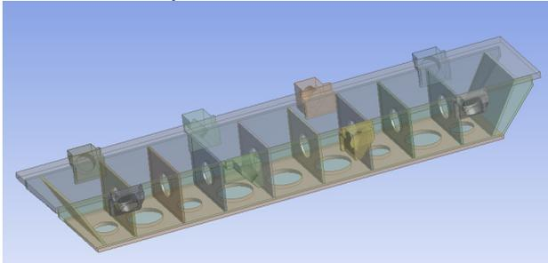
Figure 3: Structure of the girder body of Girder II.
