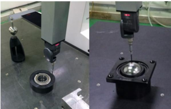
Figure 8: Calibration and test of the cam and ball transfer unit.
