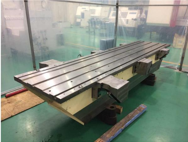
Figure 7: Girder body and ball transfer units.
