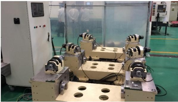
Figure 6: Pedestals and cam mechanisms.
