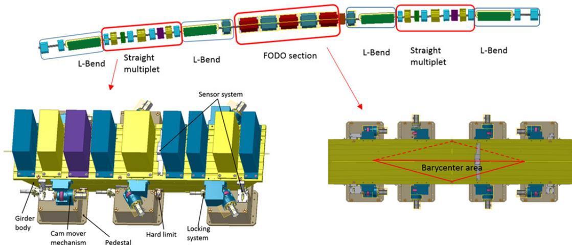
Figure 1: Overall designs of girder prototypes for HEPS-TF.
