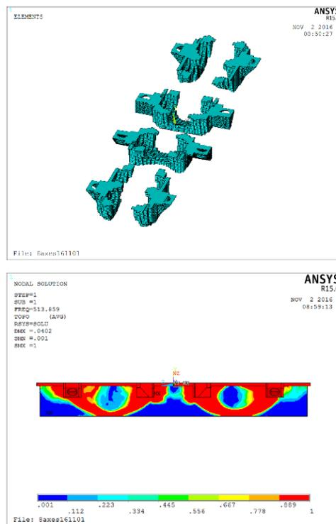
Figure 2: Topology optimization of 8-axes Girder body. U: structural optimization; D: modal optimization.
