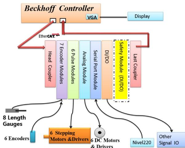
Figure 4: Control scheme of girder I.
