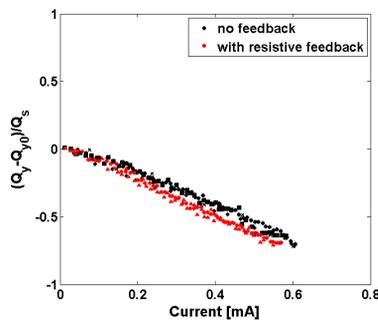
Figure 2: Normalised vertical tune shift versus single bunch current without (black) and with (red) the TMBF at zero chromaticity.
