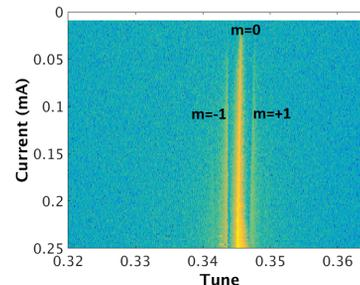
(b) With resistive feedback, maximum current at 0.25 mA.
