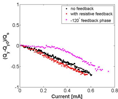
Figure 5: Normalised vertical tune shift versus single bunch current without (black) and with resistive TMBF with a phase of  $-180^\circ$  (red). A comparison is shown with an intermediate feedback phase of  $-120^\circ$  (magenta).
