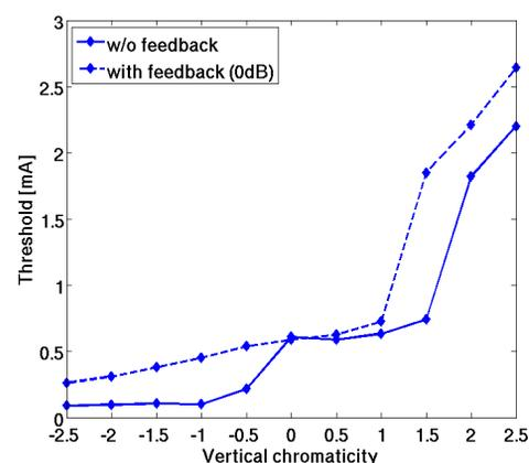
Figure 1: Vertical single bunch thresholds without and with the TMBF as a function of chromaticity.
