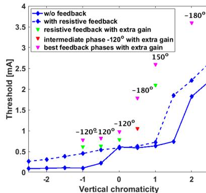
Figure 6: Vertical single bunch thresholds without TMBF (solid blue) and with nominal settings of the TMBF operating in resistive mode (dashed blue) as a function of chromaticity. In the same plot are included the measured thresholds with the TMBF with the extra gain operating in fully resistive mode (green) and at an intermediate phase of  $-120^\circ$  (red). The highest achieved thresholds are noted at each chromaticity along with the feedback phase (magenta).
