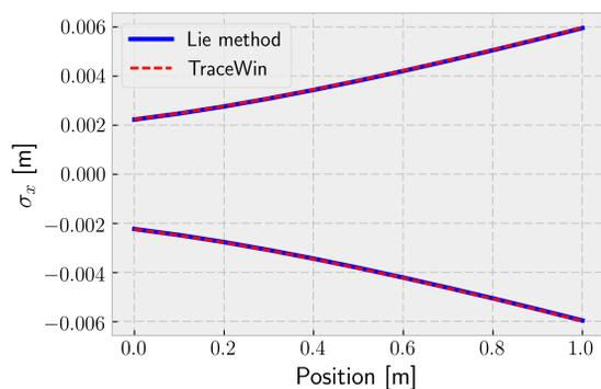
Figure 2: Beam size along 1 m drift space, calculated using Lie method (solid blue) and TraceWin (dashed red). Simulations for a 3 MeV proton beam of 50 mA with a KV distribution, a normalized emittance of  $0.1 \pi$  mm mrad and Twiss parameters  $\alpha = -1 \pi$  and  $\beta = 1 \pi$  mm / mrad.
