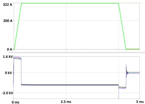
Figure 4: Important features of the simulation results are the 370  $\mu$ s rise and fall times in the current (top) and that the largest potential to ground anywhere in the system is only 1.62 kV (bottom).
