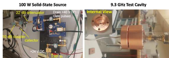
Figure 6: (left) Assembly of the three stage 100 W amplifier chain. Isolators are placed between stages. (right) 9.3 GHz cavity powered by solid-state source. The cavity is critically coupled from one side and weakly coupled from the other side using coaxial probes, loaded Q factor is 3200.
