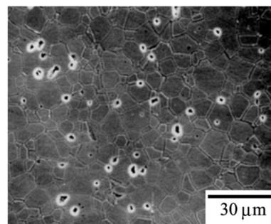
Figure 1: Typical microstructure of sintered Al<sub>2</sub>O<sub>3</sub> showing pores and grain structure [2].
