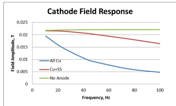
Figure 6: The interaction field response to the trim coil as a function of frequency. The blue curve represents the all Cu anode, the red curve represents the Cu+SS anode and the green curve represents the case without the anode.
