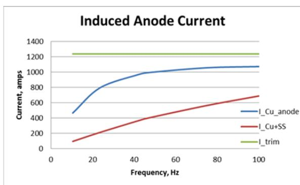
Figure 5: Current flowing in the all Cu anode (blue), the Cu+SS anode (red) and the trim coil (green) as a function of trim drive current frequency.
