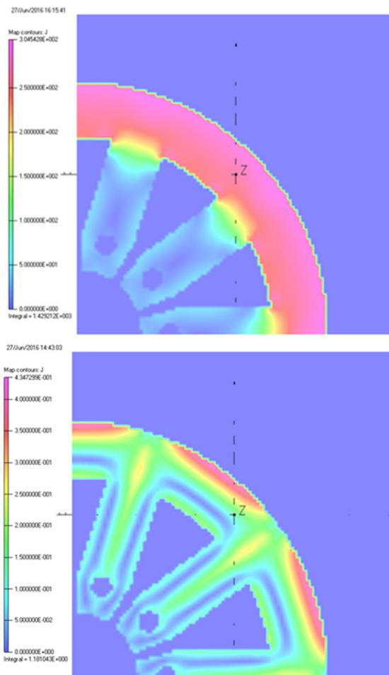
Figure 4: Contour plots of the induced Eddy current density in the anode. The upper plot (a) shows the current density without mid-vane insulation. The lower plot (b) shows the current density distribution with insulation separating the two halves of each vane along the vane radial mid-plane.
