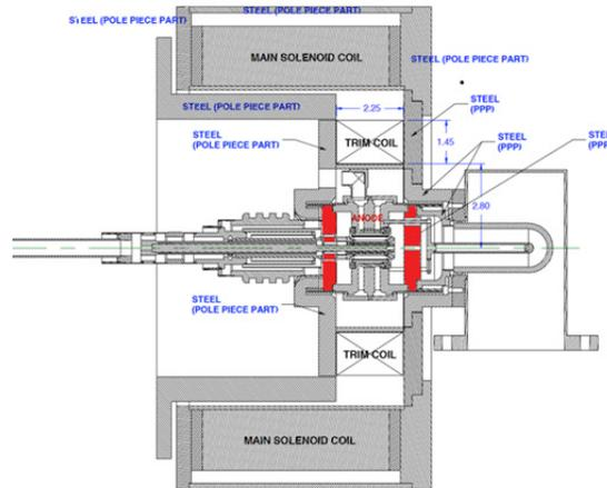
Figure 1: Diagram of the R&D magnetron showing the magnet configuration.
