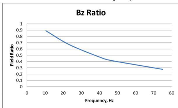
Figure 3: Ratio of interaction region field with anode eddy currents to the field without the eddy currents.
