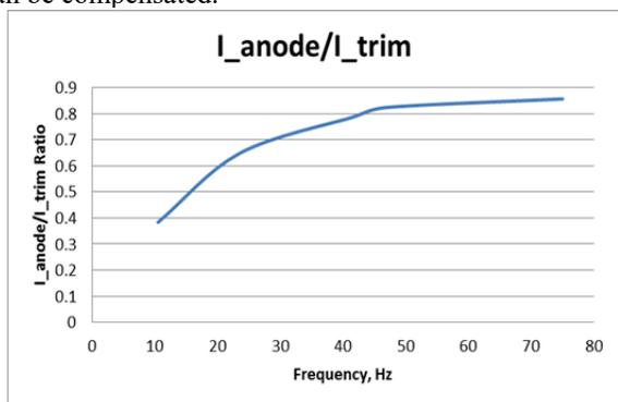
Figure 2: Ratio of eddy current in the copper anode to the trim coil current as a function of frequency.
