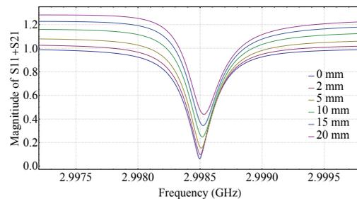
Figure 4: Simulation of  $S_{11} + S_{21}$  from the cavity to each port as port 1 input phase is varied.
