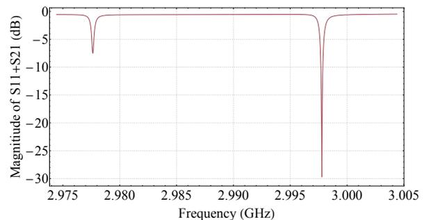
Figure 2: Measured reflection coefficient calculated from the S-parameters at both input ports at  $\frac{1}{3}$  psi positive nitrogen pressure at 50 °C.
