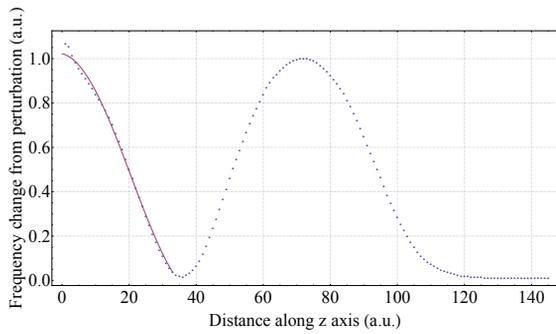
Figure 3: Bead-pull measurement of on axis field
