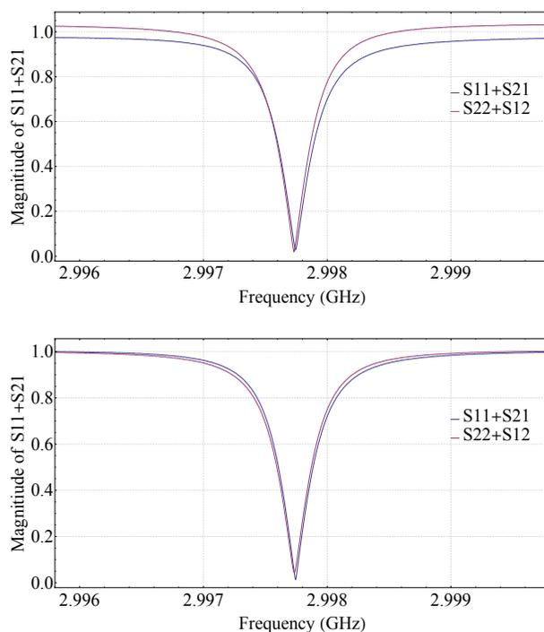
Figure 6: Reflection measurement before and after retuning.
