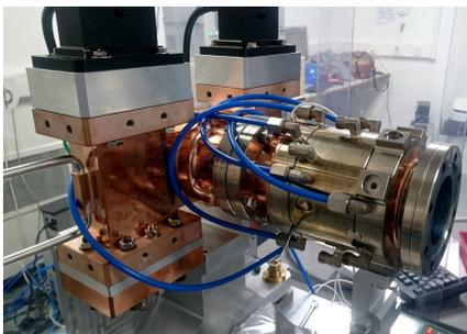
Figure 1: 400 Hz photoinjector on the bead-pull test stand at Daresbury Laboratory.
