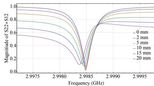
Figure 5: Simulation of  $S_{22} + S_{12}$  from the cavity to each port as port 1 input phase is varied.
