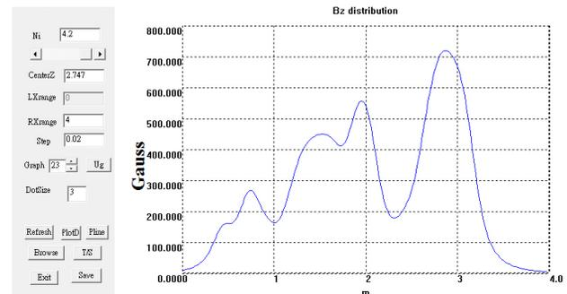
Figure 5: The Bz distribution is interactively replotting on the right while adjusting some of the coil current settings knobs on the left column.
