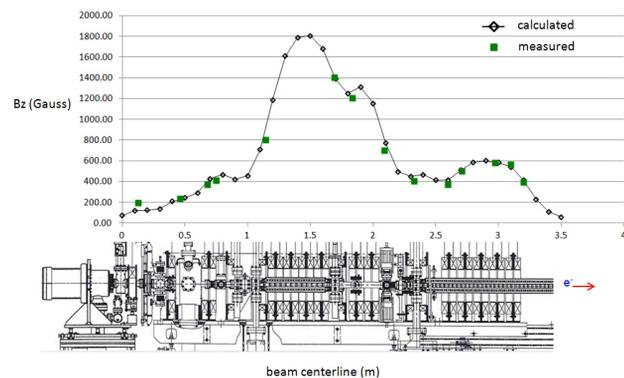
Figure 3: Comparison of the calculated and measured  $B_z$  along beam centerline.
