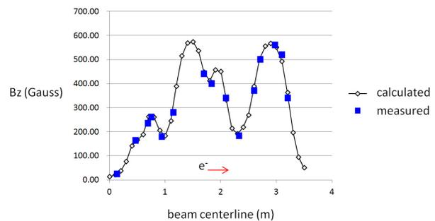
Figure 2: Comparison of the calculated and measured  $B_z$  along beam centerline.
