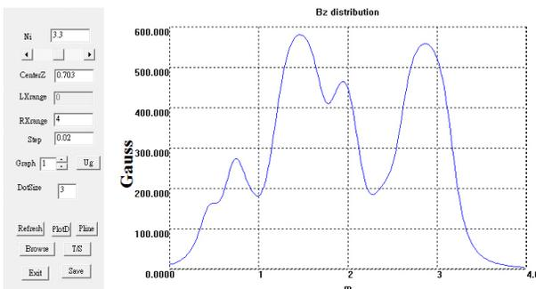
Figure 4: Typical example of the calculated Bz using the toolkit: linac\_Bz.
