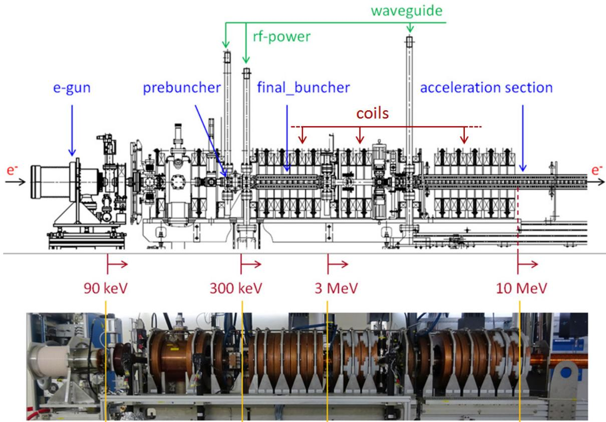
Figure 1: Layout of linac low energy region (< 10 MeV).
