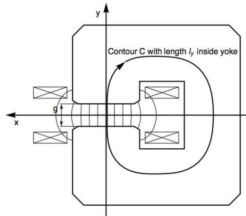
Figure 2: Transverse cross section of the magnet with an integration path to estimate the remanent field.
