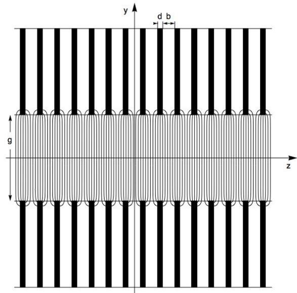
Figure 3: Magnet cross section in longitudinal direction with "thinning" of the yoke. The black rectangles denote laminations made of electrical steel interleaved with non-magnetic filling material in white (stainless steel for the ELENA prototype magnets).
