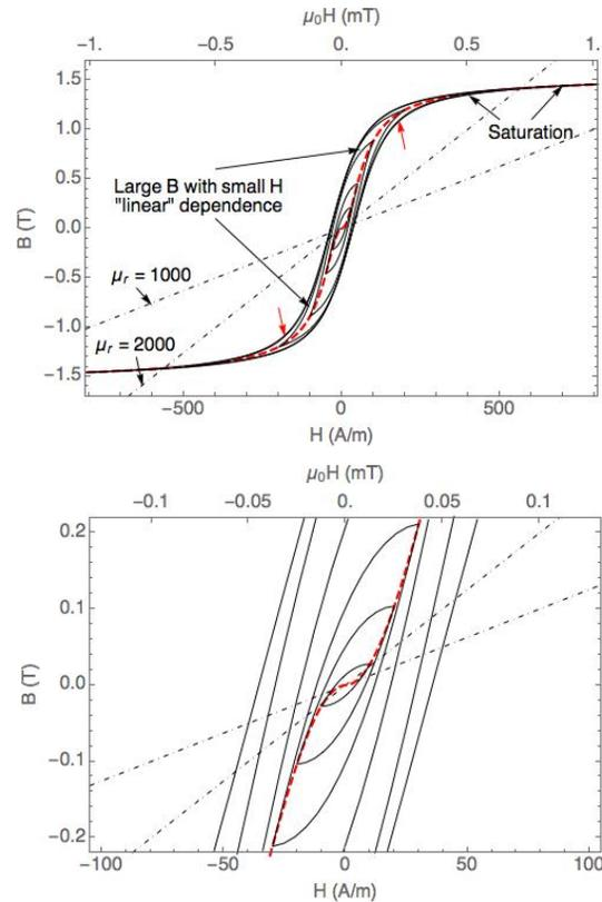
Figure 1: Hysteresis loops (solid lines) based on the formalism in Ref. [10].  $B$ - $H$ -curve as used for simulations of very low field magnets are plotted as red dashed lines. Lines corresponding to a relative permeabilities of 1000 and 2000 are shown as dot-dashed lines.
