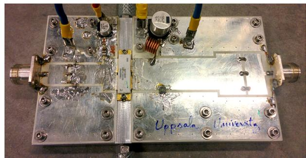
Figure 2: Kilowatt-level power amplifier in a single-ended architecture at 352 MHz.
