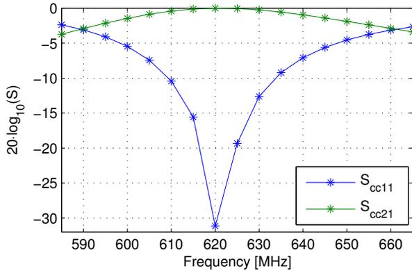
Figure 4: The simulated common-mode S-parameters of the cavity.
