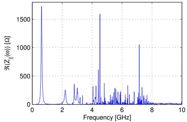
Figure 6: The longitudinal beam impedance  $\Re(Z_{||}(\omega))$  obtained in GdfidL.
