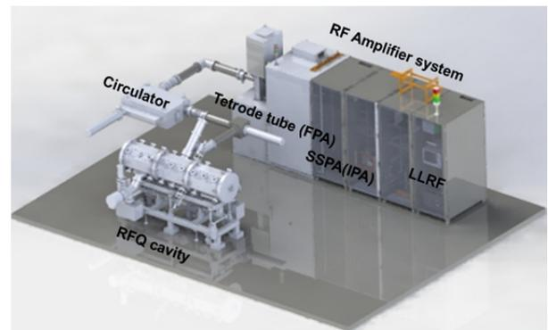
Figure 9: The photo of amplifier system for RFQ.
