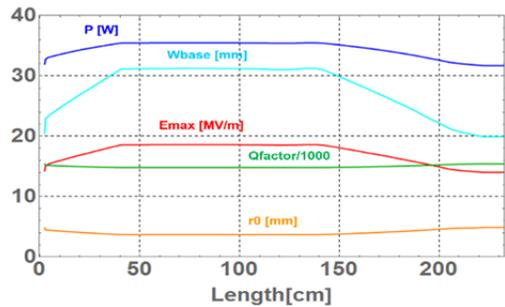
Figure 1: Power consumption in a quadrant of RFQ.
