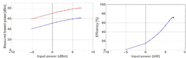
Figure 8: Result of linearity performance of FPA system.
