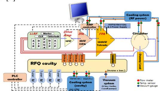
Figure 2: Diagram of RF system including the RFQ.
