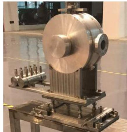
Figure 5: Prototype of prebuncher.
