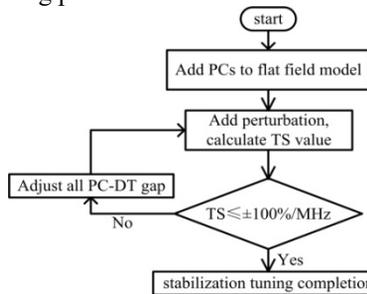
Figure 7: Process of stabilization tuning.
