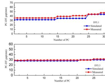
Figure 9: Comparison of simulated and measured value of PC-DT gap of DTL1 and DTL3.
