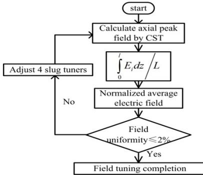
Figure 4: Procedure of field tuning.
