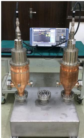
Figure 8: The manufactured power-conditioning cavity connected with two coaxial power couplers in measurement.
