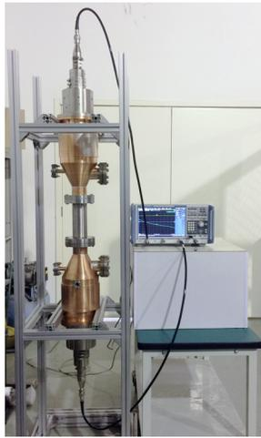
Figure 3: Couplers connected with converters in measurement.
