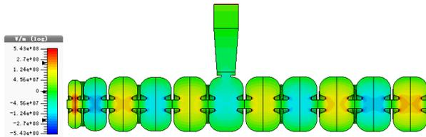
Figure 3: E-field along the axis of the structure.
