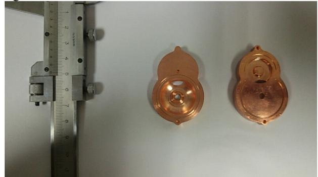
Figure 6: Single cell before welded.
