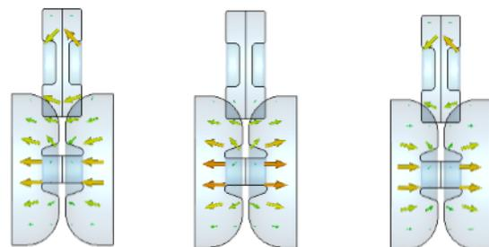
Figure 2: E-fields of 0 mode (left),  $\pi/2$  mode (middle) and  $\pi$  mode (right)
