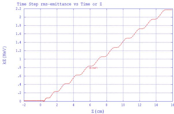
Figure 4: Particle energy along the structure.
