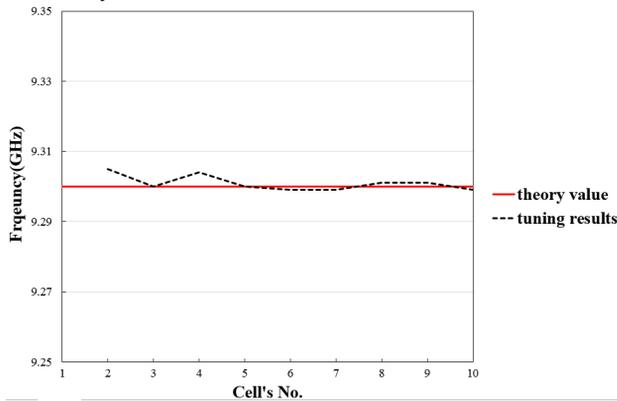
Figure 8: Measurement results compared with theory value.
