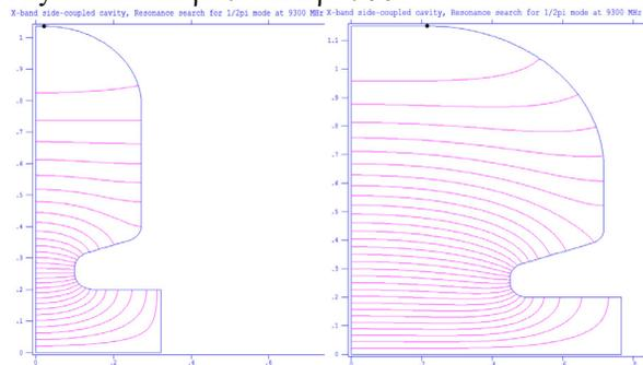
Figure 1: Accelerating cells  $\beta=0.4$ (left) and  $\beta=0.95$ (right).
