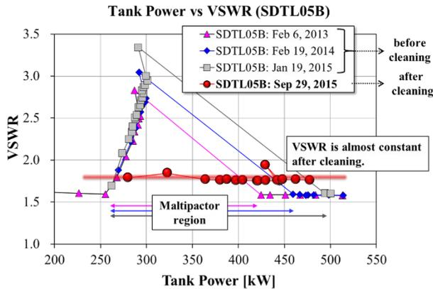
Figure 5: VSWR as a function of tank power before and after cleaning (SDTL05B).
