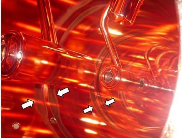
Figure 2: Photograph of inside view of SDTL05B. The arrows show the discolored bands.
