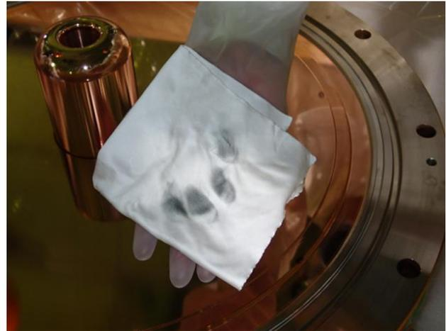
Figure 4: Wiping cloth after wiping inner surface of end plate of SDTL05B.
