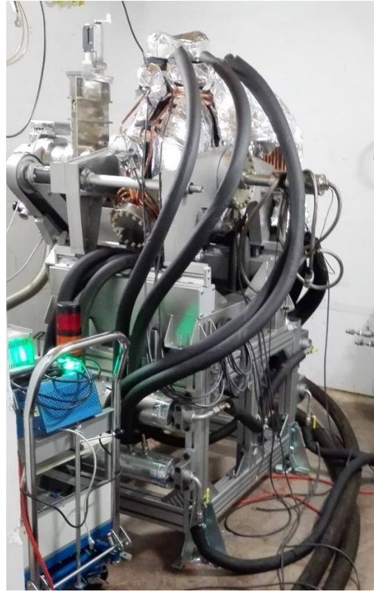
Figure 5: Indus-2 Cavity during the bake out.
