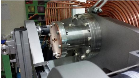
Figure 3: Cavity bead pull measurement with the additional pipes along the beam axis.
