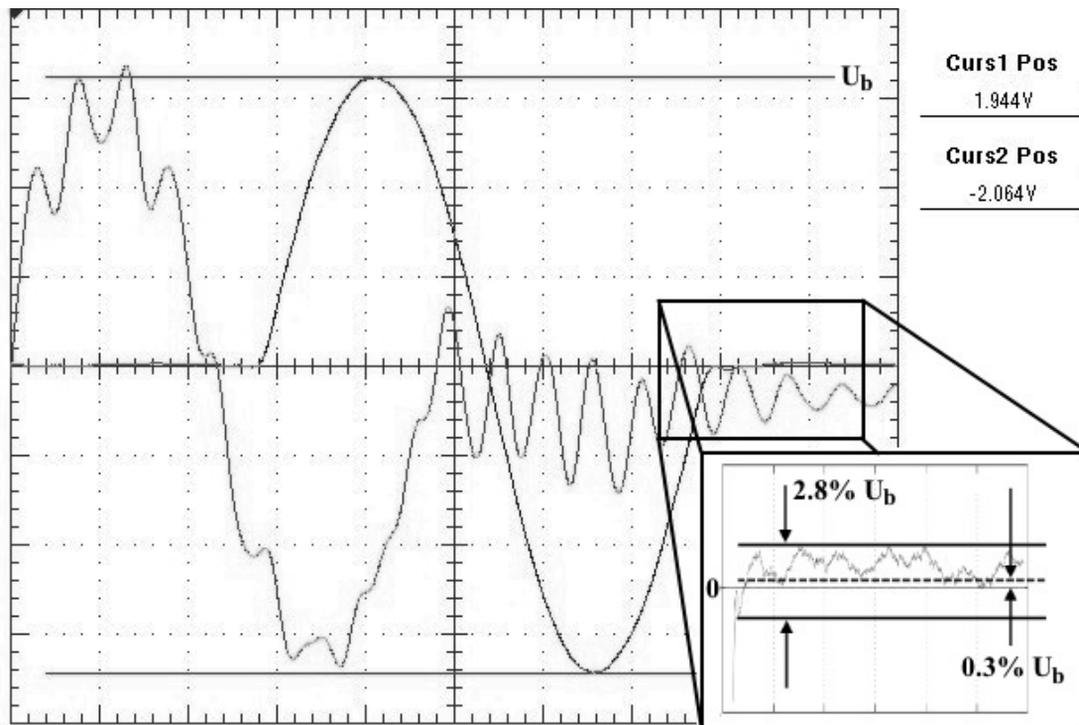
Figure 7: Input signal (jagged line) and single-sine barrier pulse at the output port of a 1:800 gap voltage divider.
