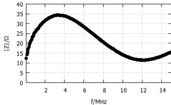
Figure 4: Magnitude of amplifier load impedance  $Z$ .
