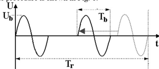
Figure 1: Barrier pulses of duration  $T_b$  and amplitude  $U_b$  are shifted towards each other to compress the beam revolving with period  $T_r$ .
