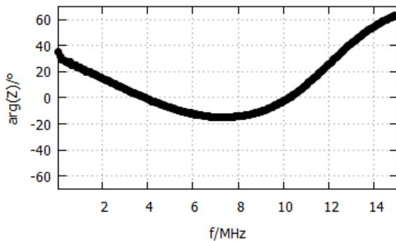
Figure 5: Phase of amplifier load impedance  $Z$ .
