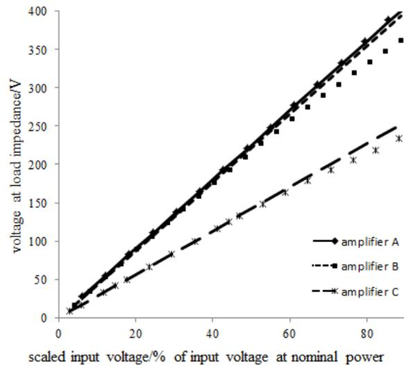
Figure 6: Voltage characteristics for three different amplifiers. Considerable non-linearity is observed for amplifiers B and C, thus only a fraction of their nominal power can be used for generation of Barrier-Bucket pulses with pre-distortion based on Fourier analysis.
