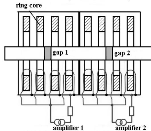
Figure 2: In each cavity box, one RF pulse per revolution is generated. Two cavity boxes share one housing.
