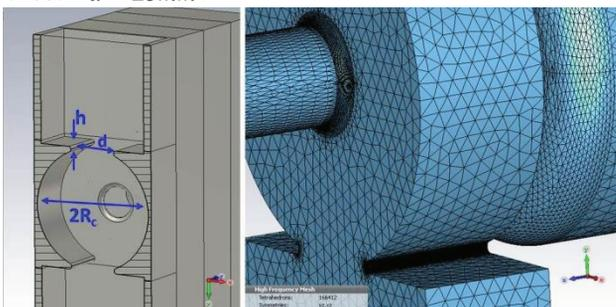
Figure 4: Coupler geometry and mesh.
