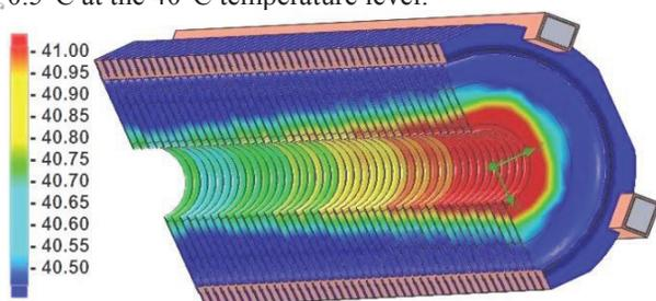
Figure 9: Temperature gradient along TW structure.
