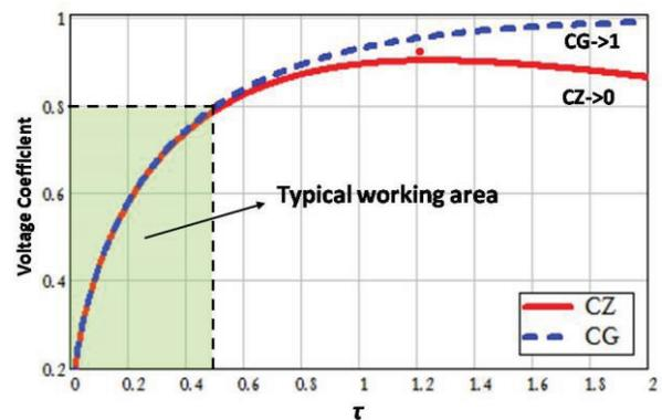
Figure 1: Voltage coefficient for constant gradient (CG) and constant impedance (CZ) accelerating structures.
