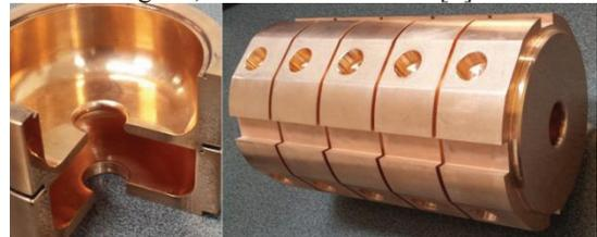
Figure 10: Brazing test with 2-cell (left) and 5-cell prototypes (right).
