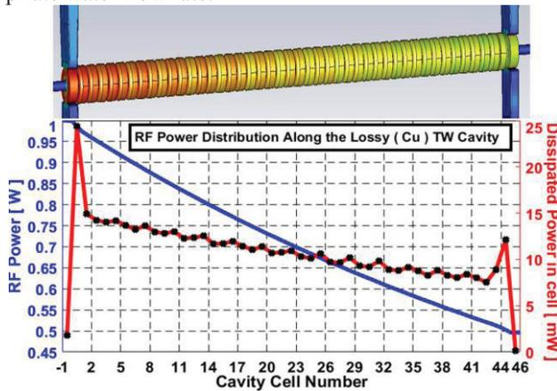
Figure 8: Propagated and dissipated power distributions along the lossy TW cavity.
