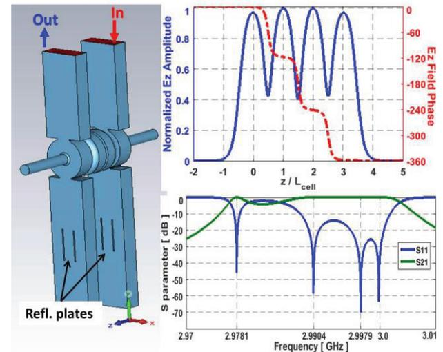
Figure 6: Reduced cavity model: TW accelerating field and S parameters.
