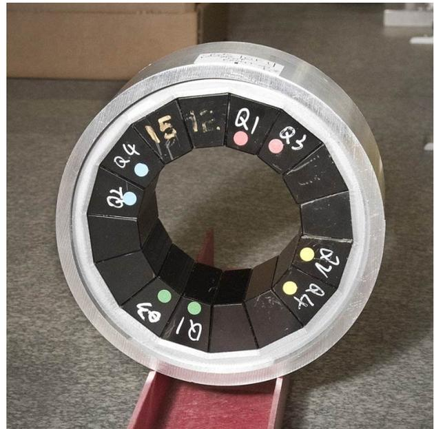
Figure 3: QF magnet without iron wires.
