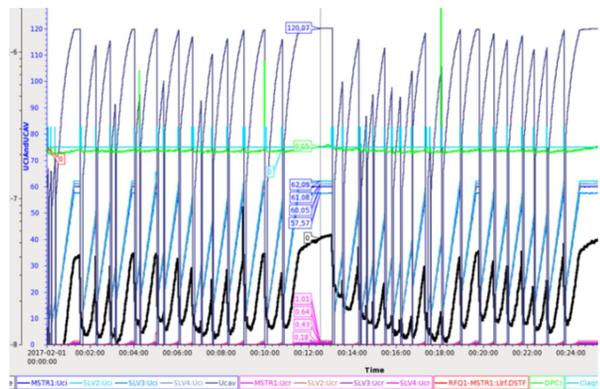
Figure 5: RF conditioning with frequency follow system.
