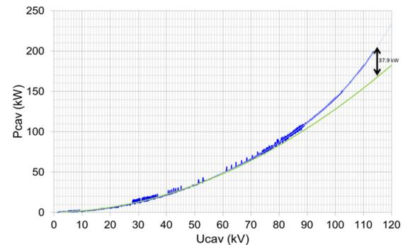
Figure 8: Cavity voltage according injected power.
