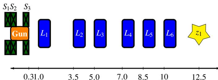
Figure 1: Layout of the AWA linac. The gun is enlarged to show solenoid detail. The physical length is 0.3 m. The cathode is located at  $z = 0$  m. Linac cavities are 0.85 m long. Tick marks are located at the exit of the gun, entrance of each accelerating cavity, and location of optimization.
