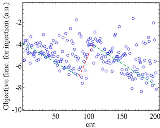
Figure 3: Objective function during injection optimisation from the HBT to the storage ring.
