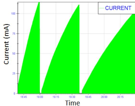
Figure 4: Beam current in the storage ring.
