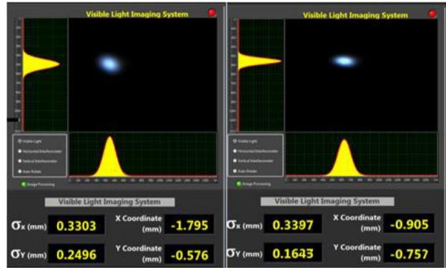
Figure 6: Visible light beam profile before (left) and after (right) RCDS optimization.
