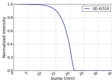
Figure 2: Intensity evolution during the scan of the amplitude of a three-corrector bump at location of QD.42510.
