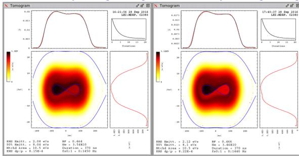
Figure 4: Almost-identical tomograms for an  $h=2+4$  beam achieved with one (left) and two (right) HLRF systems.
