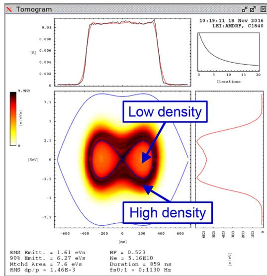
Figure 5: Hollow bunch after capture, showing a remarkably flat profile.
