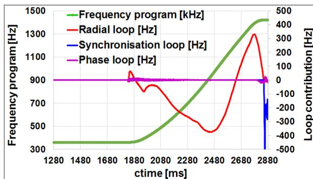
Figure 2: Frequency program (left axis) and loop contributions (right axis) for a Pb<sup>54+</sup> NOMINAL cycle.
