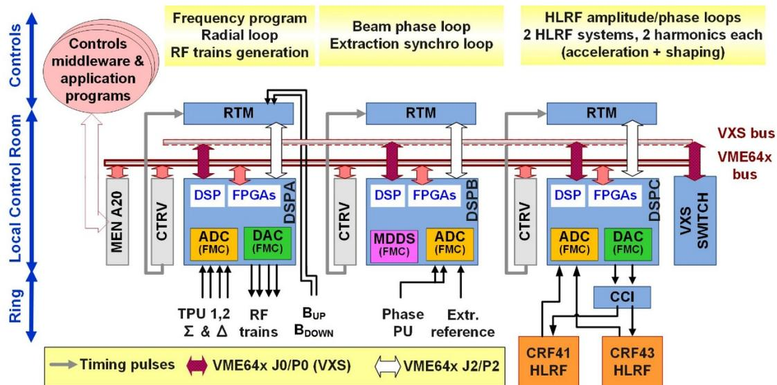
Figure 1: LEIR LLRF schematic view. Keys: MDDS – Master Direct Digital Synthesiser; ADC – Analogue-to-Digital Converter; DAC – Digital-to-Analogue Converter; TPU – Transverse Pick-up; CTRV – Timing Receiver Module; MEN A20 – Master VME board; RTM – Rear Transition Module; CCI – Cavity Control Interface.
