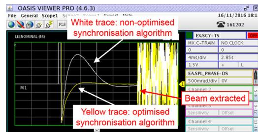
Figure 3: Beam-to-extraction reference phase signals during the extraction synchronisation loop. White trace: non-optimised algorithm. Yellow trace: optimised algorithm.
