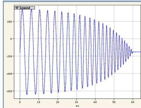
Figure 6: Modulated frequency offset function during the first 60 ms of the beam capture process.
