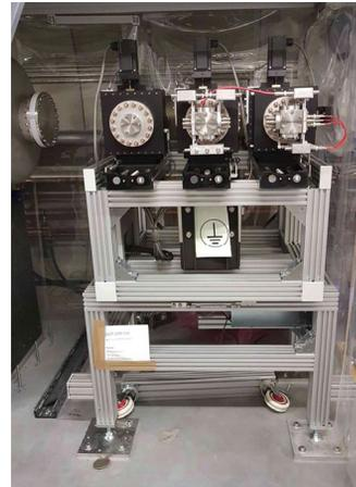
Figure 5: SASE3 MCP detector in XFEL tunnel.
