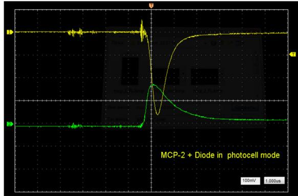
Figure 3: MCP2 and photo diode signals produced by flash lamp.
