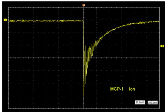
Figure 4: MCP1 signal from an ion produced in the ion pump.
