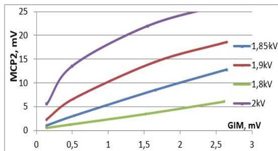
Figure 1: Dependence of MCP2 signal on gas ionization chamber signal at different MCP 2 voltages.
