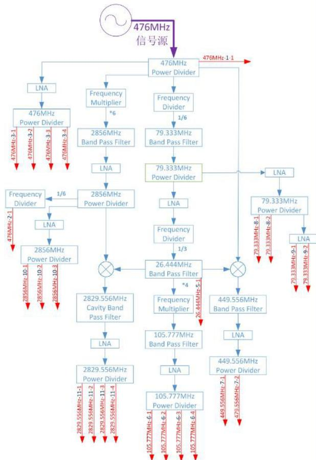
Figure 2: Structure of frequency distribution system.
