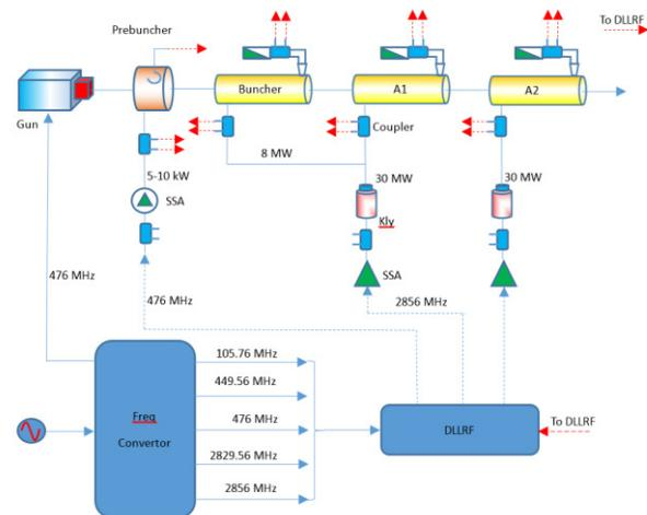
Figure 1: Structure of microwave system of IR-FEL.
