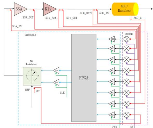
Figure 4: Signal transmission of LLRF.
