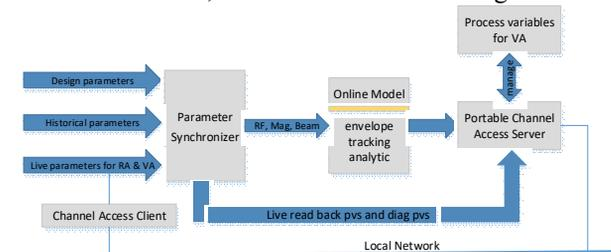
Figure 4: Schematic view of virtual accelerator for XiPAF.
