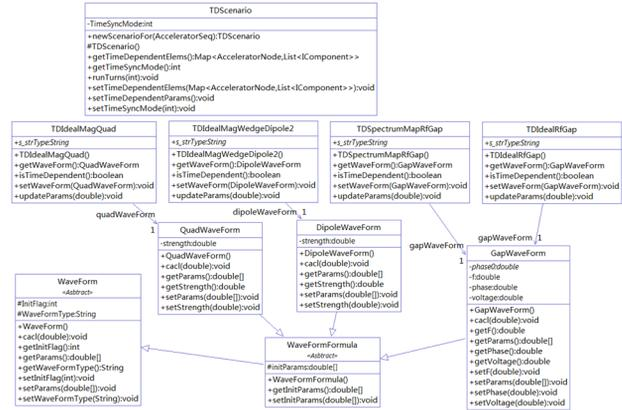
Figure 5: Class diagram of classes related to ramping simulation.
