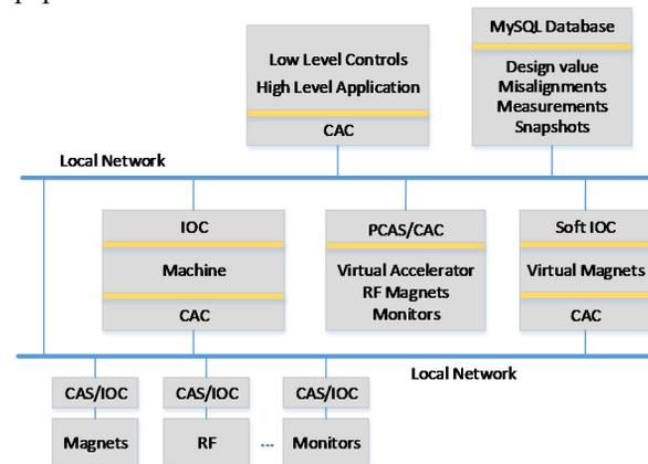
Figure 1: Schematic layout of EPICS control system and high-level controls based on Open XAL for XiPAF.
