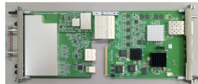
Figure 3: Photo of a new digitizer AMC and a signal conditioning RTM.
