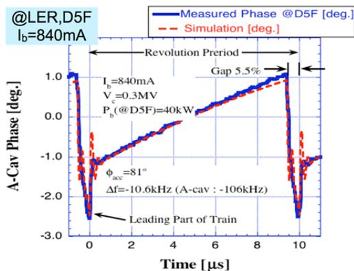
Figure 5: RF phase modulation in the accelerating cavity of ARES (blue line), which was measured by new LLRF control system in Phase-1, and the simulation result are plotted together during the revolution period (dashed line).
