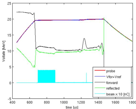
Figure 1: Calibrated forward and reflected voltages at cav.1 ACC1 at FLASH. Additionally the FLASH1 and FLASH2 beams are shown for reference.
