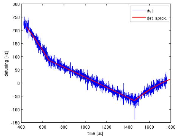
Figure 2: Detuning and its approximation for RF and beam signals from figure 1. The beam contribution is calibrated and taken into account.
