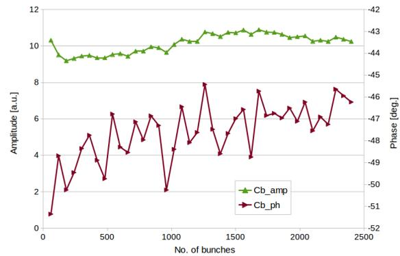
Figure 3: Dependency of calibration factors on beam intensity. Measurements were done at cav.1 ACC6 during "9mA" experiments. Beam current 4.5 mA, number of bunches variable in the range from 60 up to 2400 (3 MHz, 1,5 nC).
