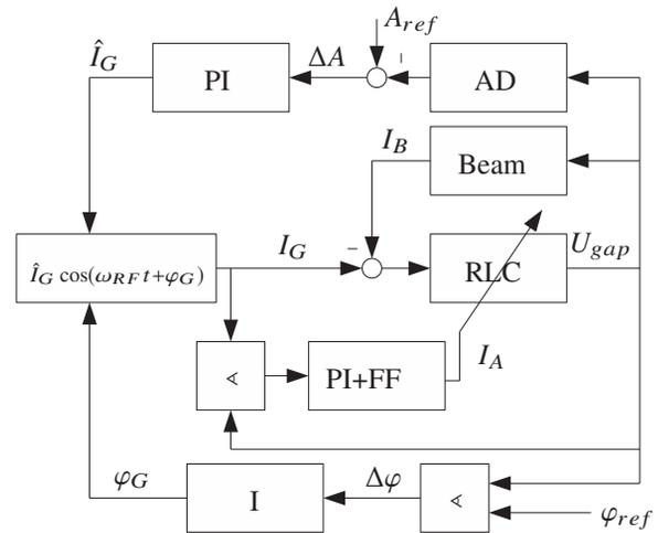
Figure 1: Block diagram of cavity and beam dynamics with control loops.
