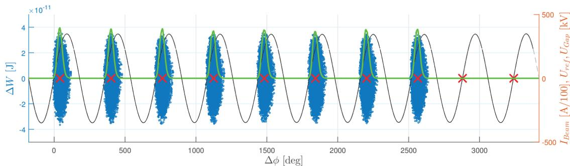
Figure 3: Complete bunch train during acceleration: particles (blue), beam current (green), gap voltage (black) and center of gravity (red).
