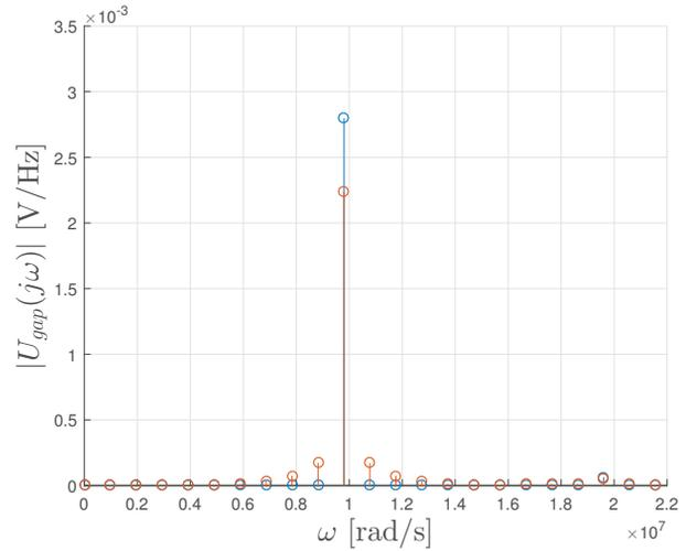
Figure 2: Magnitude spectrum response of the cavity to a beam current with unity amplitude: Ten filled buckets (blue), eight out of ten filled buckets (red).
