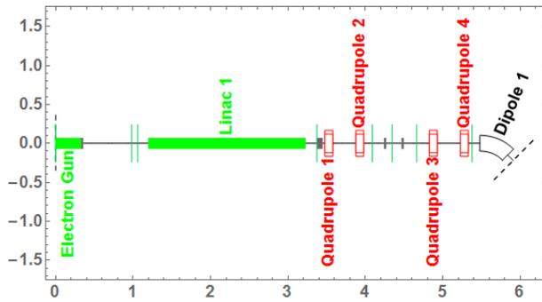
Figure 1: Schematic diagram of the CLARA beamline section used in the simulations. Also included is a solenoid located at the electron gun, combined with a bucking coil to reduce the solenoid field to zero at the photocathode.
