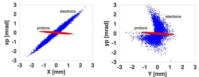
Figure 6: Transverse phase space of the imported electron bunch distribution, which was generated by PTC tracking simulations of the electron beam line.
