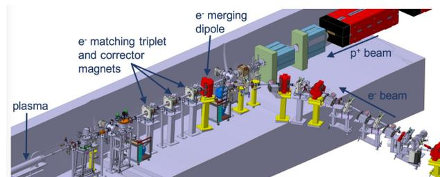
Figure 1: View of the AWAKE primary beam lines upstream of the plasma cell. The e- merging dipole bends the electron beam onto the proton beam axis. The final focussing quadrupoles of the electron beam are located between the merging dipole and the plasma cell. Additional corrector magnets can be used to introduce an offset between the two beams.
