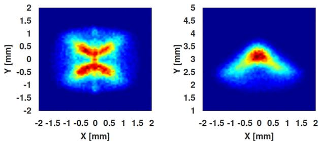
Figure 5: The transverse profiles of the electron bunch at the focal point after propagation through the common beam line on-axis (left) and with an offset of 3 mm between the electron beam axis and the proton beam axis (right).
