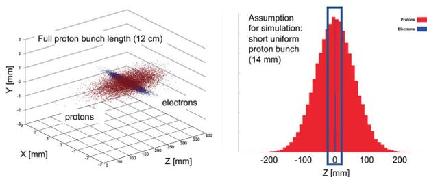
Figure 2: Starting distribution of the electron and proton bunch from the optics TWISS parameter. The long gaussian proton bunch has been reduced in the simulation model to a short one around the electron bunch with a constant particle distribution as indicated by the window in the histogram.
