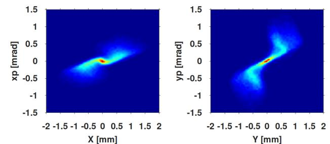
Figure 4: The electron phase space at the focal point after copropagation on axis with the  $3 \cdot 10^{11}$  proton bunch.
