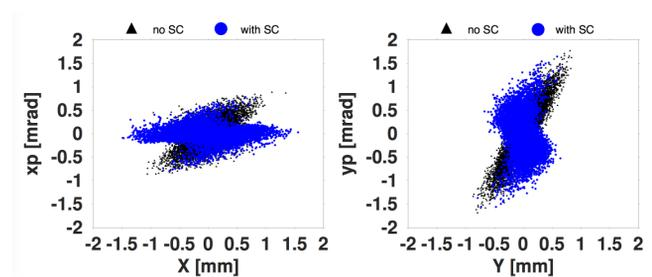
Figure 3: The electron phase space at the focal point with and without space charge included in the tracking algorithm.
