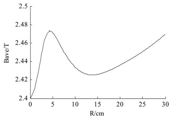
Figure 6: Radial distribution of the average magnetic field in central region.
