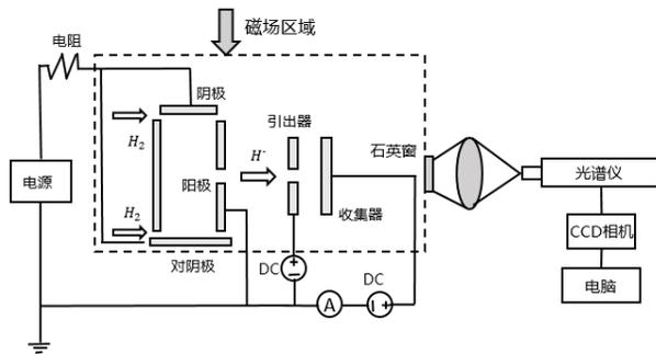
Figure 3: Schematic diagram of the central region electrode.
