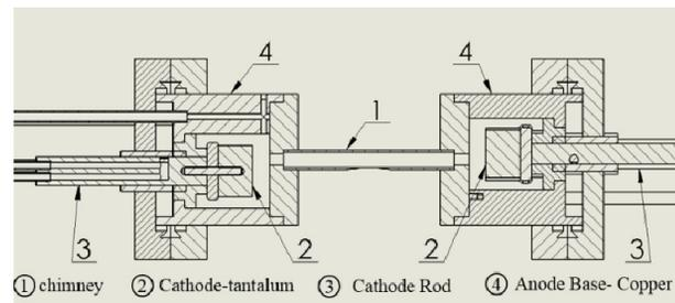
Figure 1: Structure diagram of the PIG source.
