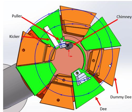
Figure 4: Structure diagram of the central region electrode.
