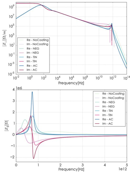
Figure 1: Real and imaginary part of the transverse (top) and longitudinal (bottom) RW impedances as a function of the frequency in the case of no coating, NEG coating, TiN coating and Carbon coating.
