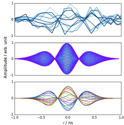
Figure 4:  $Q' = 9$ , measurements from the LHC head-tail monitor signal (top), PyHEADTAIL simulations (middle) and DELPHI simulations (bottom).
