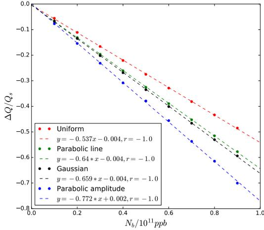
Figure 2: Real part of the most unstable mode frequency shift, normalised by the synchrotron tune, as a function of single bunch intensity (in protons per bunch).
