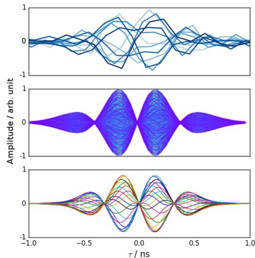
Figure 5:  $Q' = 15$ , measurements from the LHC head-tail monitor signal (top), PyHEADTAIL simulations (middle) and DELPHI simulations (bottom).
