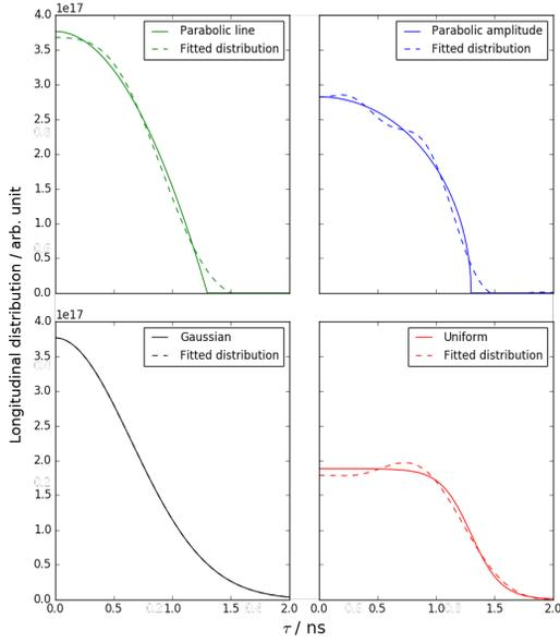
Figure 1: Longitudinal particle distributions as a function of length in ns. Four distributions are showed: parabolic line, parabolic amplitude, Gaussian and approximated uniform. The solid line shows the distribution from [4]. The dashed line show the distribution after the decomposition over Laguerre polynomials.
