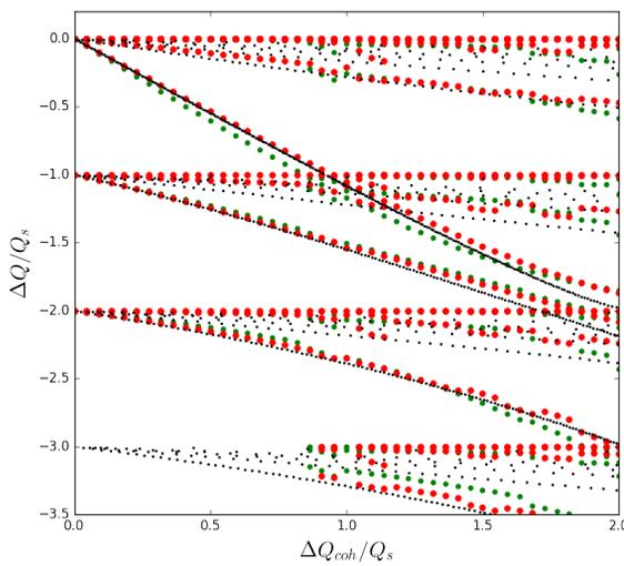
Figure 3: Real part of the modes frequency shifts obtained with DELPHI using a Gaussian longitudinal distribution (green), an uniform distribution (red), compared to Laclare formalism (uniform distribution, black) as a function of normalised beam intensity, for a constant inductive impedance. Results are normalised by the synchrotron tune.
