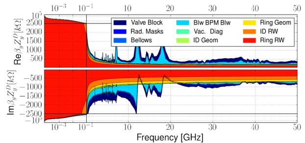
Figure 5: Vertical impedance budget weighted by the  $\beta_y$ .
