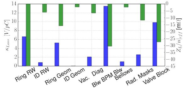
Figure 4: Single bunch loss factor  $\kappa$  (blue) and effective  $Z/n$  (green) calculated for a 3 mm bunch.
