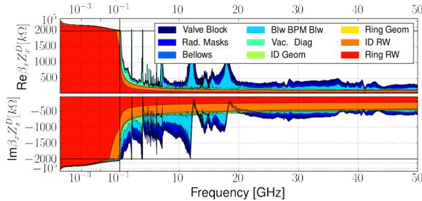
Figure 7: Vertical impedance budget weighted by the  $\beta_x$ .
