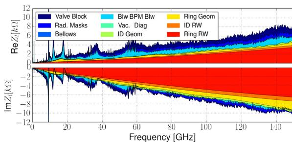
Figure 3: Longitudinal Impedance Budget for Sirius.
