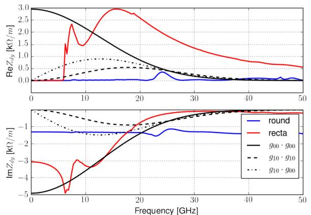
Figure 2: Vertical dipolar impedance comparison for round and rectangular transitions simulated in ECHO2D with same transition slope and vertical gap.
