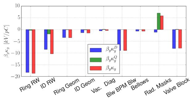
Figure 6: Single bunch vertical kick factor weighted by the  $\beta_y$  for a 3 mm bunch.
