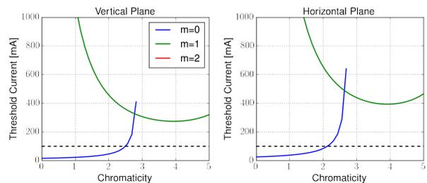
Figure 10: Uniform filling coupled bunch head-tail modes 0, 1 and 2 thresholds as function of chromaticity. The black dashed line is the nominal current of the ring.
