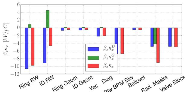
Figure 8: Single bunch horizontal kick factor weighted by the  $\beta_x$  for a 3 mm bunch.
