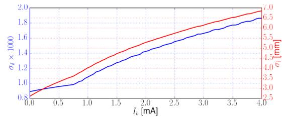
Figure 9: Bunch lengthening and energy spread predicted for Sirius as function of the single bunch current, considering IBS and longitudinal impedance.
