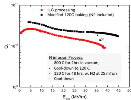
Figure 10: “Nitrogen infusion” process demonstrated at Fermilab, resulting in high-Q and high-G.
