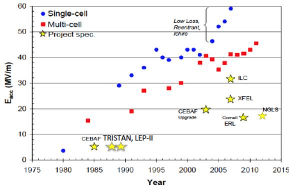
Figure 6: Progress of field gradient in single and multicell SRF cavities.
