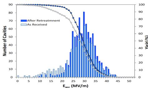
Figure 8: Field gradient distribution for the European XFEL cavities from their individual test.
