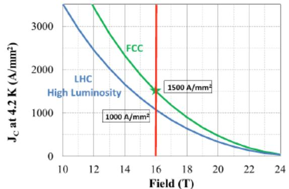
Figure 3: Critical current density improvement required for 16 accelerator magnets to be realized for Future Circular Collider (FCC).
