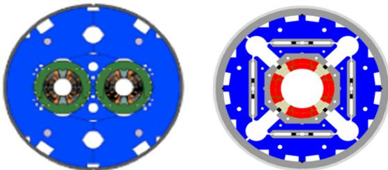
Figure 2: Cross sections of a 11 T dipole and an IR quadrupole with Nb<sub>3</sub>Sn conductor for the HL-LHC.
