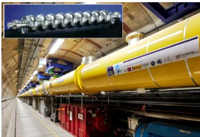
Figure 7: The European XFEL accelerator with 1.3 GHz superconducting 9-cell cavities.
