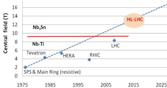
Figure 1: Progress in dipole field with NbTi superconductor for collider accelerators, and the prospect with the Nb<sub>3</sub>Sn superconductor.
