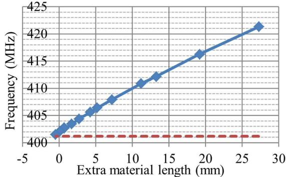
Figure 3: Frequency evolution during trim tuning for one of the prototypes. The red dashed line corresponds to the target frequency for the clamped DQW assembly.
