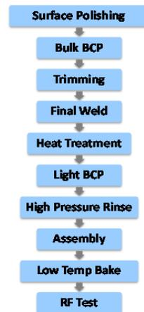
Figure 6: Sequence of cavity processing.
