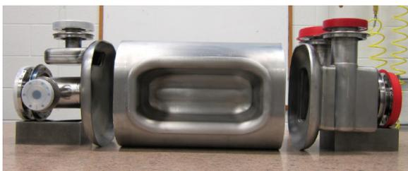
Figure 4: Sub-assemblies of rf-dipole prototype cavity.
