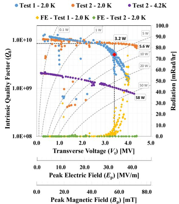
Figure 10: Quality factor at 4.2 K and 2.0 K of the 400 MHz rf-dipole cavity.
