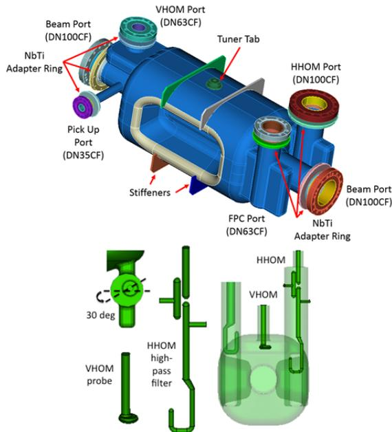
Figure 3: Bare prototype cavity for SPS (top) and FPC and HOM couplers (bottom) of the rf-dipole cavity.
