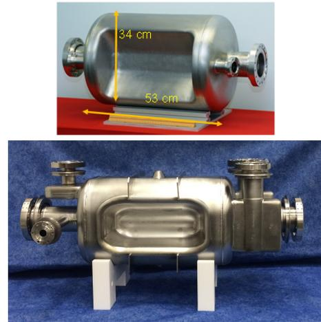
Figure 2: 400 MHz proof-of-principle (top) and prototype (bottom) rf-dipole cavities.
