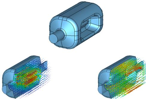
Figure 1: 400 MHz rf-dipole cavity (top) and electric (bottom left) and magnetic (bottom right) field profiles of the cavity.
