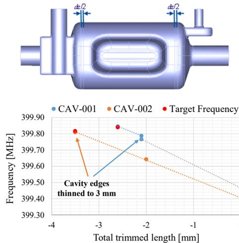
Figure 8: Trimming of Bulk BCP of sub-assemblies.
