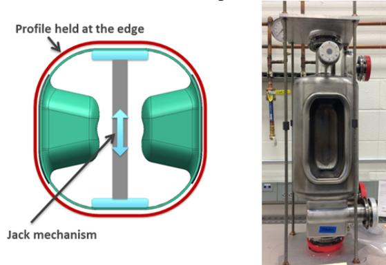
Figure 5: Set up for fixing of the center body (left) and vertical stacked assembly for frequency measurements (right).
