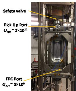
Figure 9: Cavity rf test assembly.
