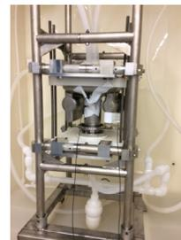
Figure 7: Bulk BCP of sub-assemblies.
