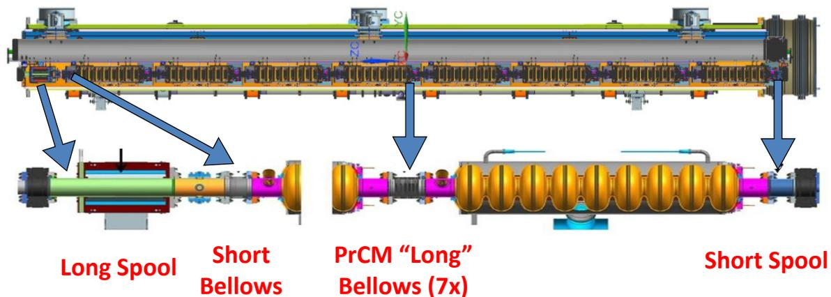
Figure 1: Location of beamline bellows and spools in the LCLS-II cryomodule.
