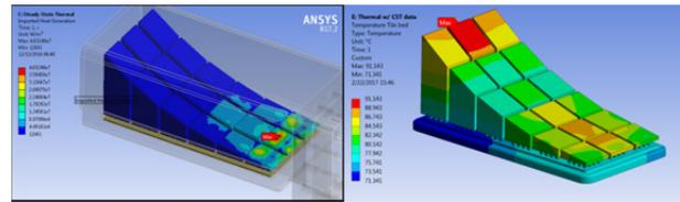
Figure 10: Left: absorber RF loss density rendered in ANSYS by superposing CST results; Right: absorber temperature simulated in ANSYS.
