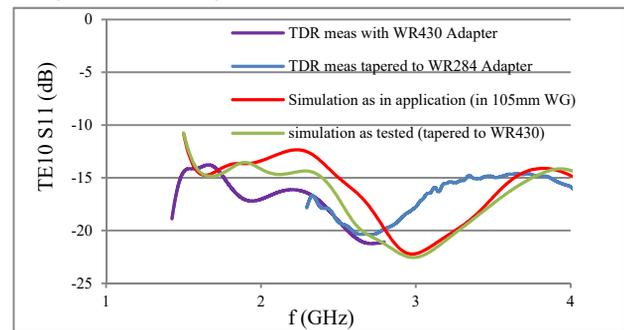
Figure 6: Network analyzer measurement of bERLinPro HOM load.
