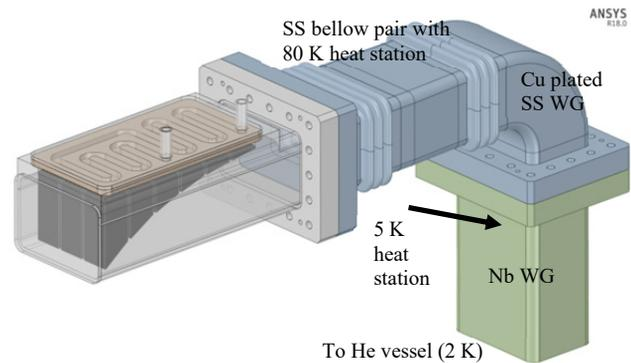
Figure 11: VSR 1.5 GHz HOM waveguide assembly.
