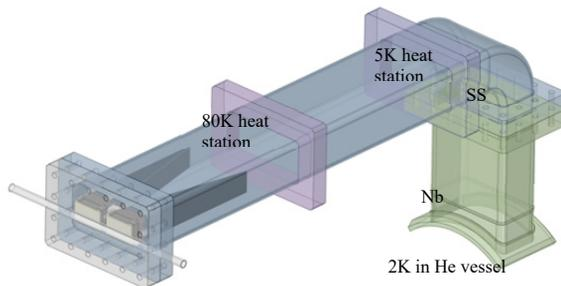
Figure 4: bERLinPro HOM waveguide assembly.
