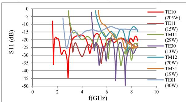
Figure 9. Return loss of VSR 1.5GHz cavity HOM load simulated in CST.
