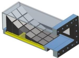
Figure 8: VSR 1.5GHz cavity HOM load design.
