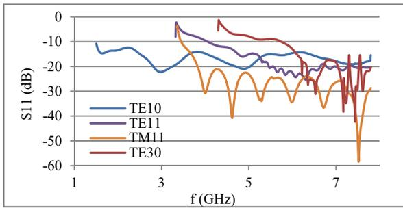
Figure 2: Simulated return loss of the bERLinPro HOM load with two 178 mm STL-100HTC wedges.
