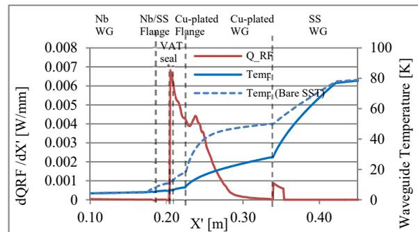
Figure 12: VSR 1.5 GHz HOM waveguide 1-D thermal optimization results.
