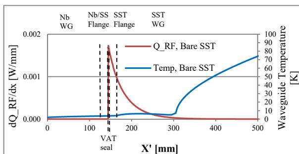
Figure 5: bERLinPro HOM waveguide 1-D thermal optimization results.
