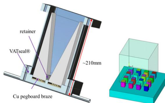
Figure 1: Left: model of the bERLinPro HOM load; Right: “pegboard” brazing concept.
