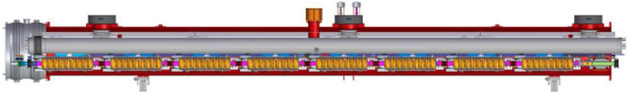
Figure 2: The LCLS-II 1.3 GHz Cryomodule.
