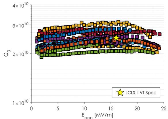
Figure 4: The Q vs. E curve for the 16 first article cavities from RI.
