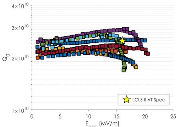
Figure 3: The Q vs. E curve for the first article cavities from EZ.
