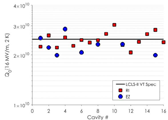
Figure 6: The  $Q_0$  measured at 16 MV/m for each of the first article cavities that were tested from the 2 vendors.
