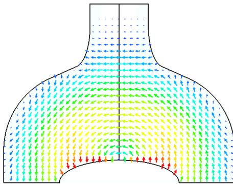
(a) The electric field pattern x-z plane.
