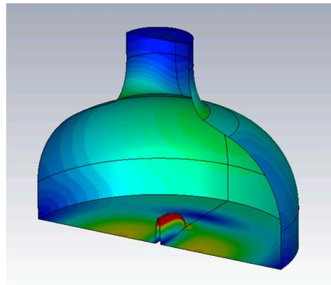
(a) Surface magnetic field magnitude. The scale has been adjusted so that field pattern off the sample is visible.
