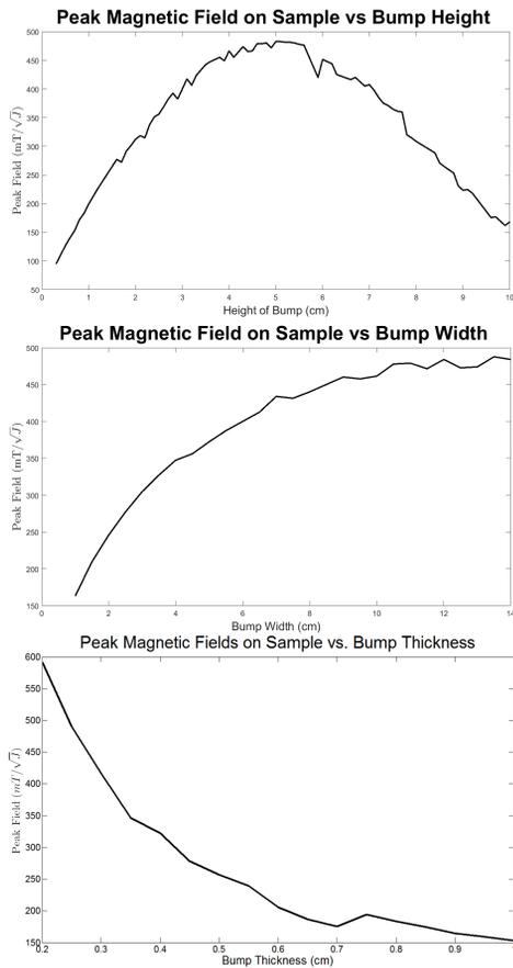
Figure 2: Peak surface magnetic field on sample for 1 J in the cavity. In each plot the unlisted dimensions are Height = 3 cm, Width = 6 cm, and Thickness = 0.3 cm. There is some noise in simulated data due to meshing.
