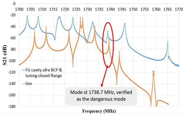
Figure 3: Simulation and measurement result comparison around 5th machine line at 300 K.
