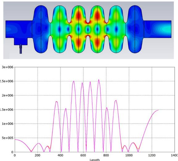
Figure 2: (Upper) simulated E-field concentration in cavity for mode at 1742 MHz; (lower) its simulated E-field profile on cavity axis.
