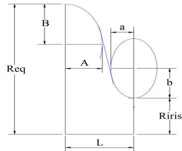
Figure 1: Schematic of 7 independent geometrical dimension in an elliptical cavity.
