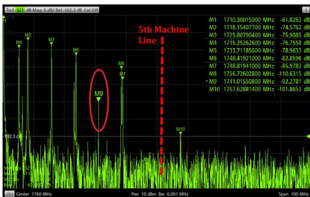
Figure 5: 6-cell cavity with FG Nb HOM measurement result at 2K with tank around 5th machine line.
