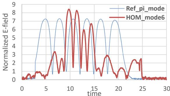
Figure 4: E-Field profile measured on cavity axis by bead-pulling for mode at 1738.7MHz at 300 K.
